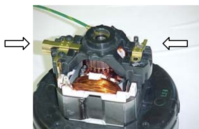
Fig 2: 1 Motor Brush Removed
