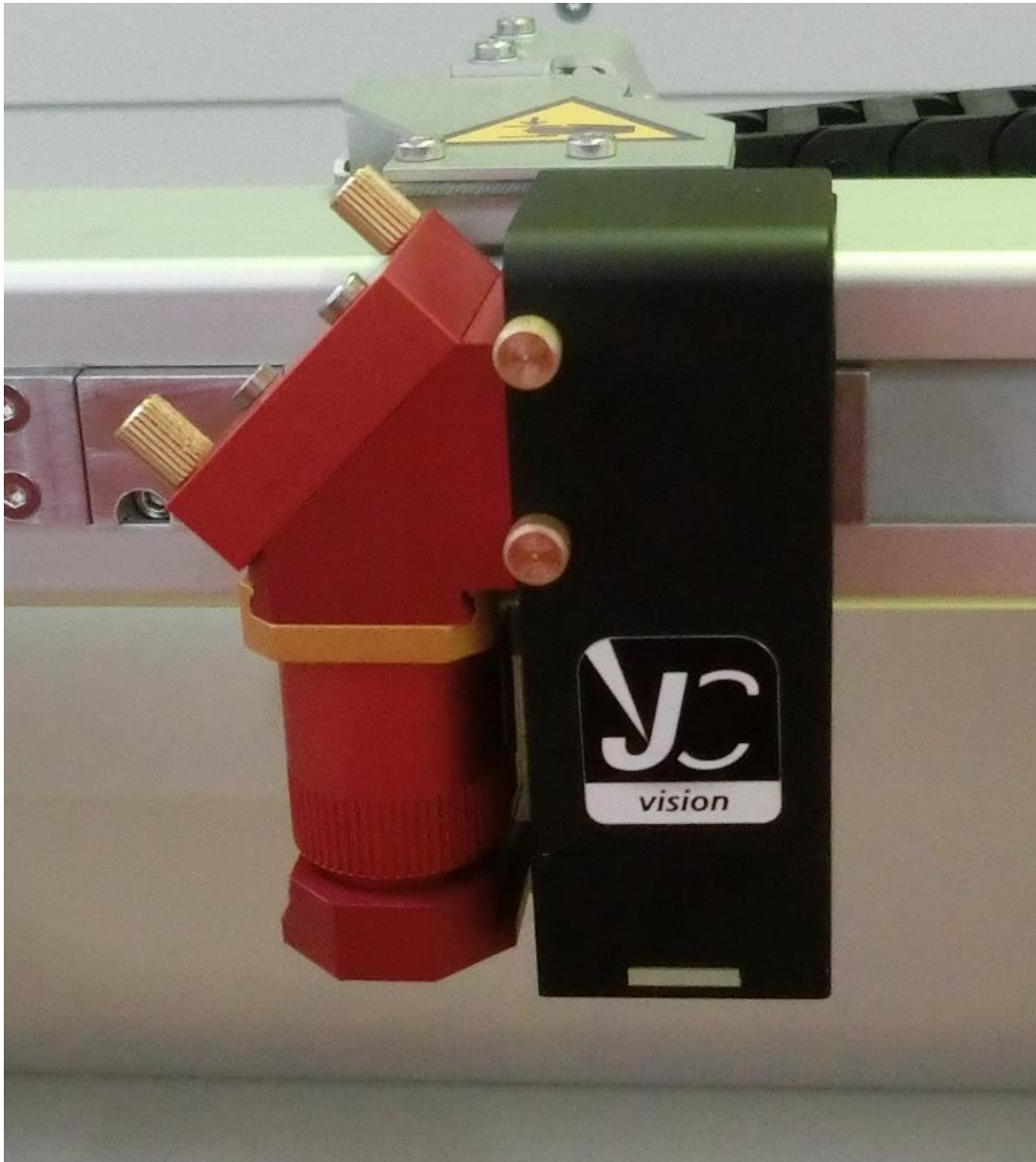
JobControl ® Vision Camera system with LED/protection adapter.
