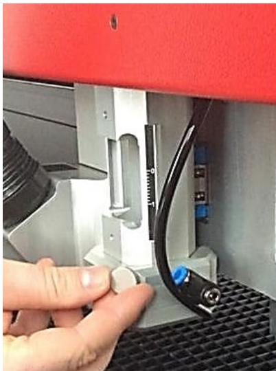
4. Retirez la vis de fixation. (1 vis)
