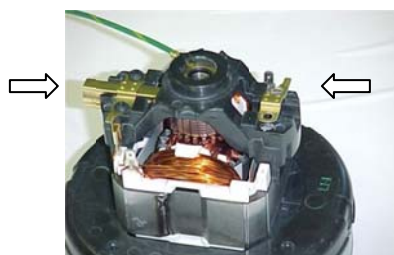
Fig 2: 1 Motor Brush Removed
