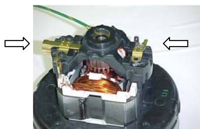
Fig 2: 1 Motor Brush Removed
