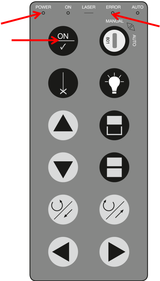
Figure 5: Laser workstation front panel of SpeedMarker 700 and 1300
