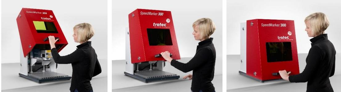
Simply use the black handle at the door to lift it and slide it down for opening and closing.
